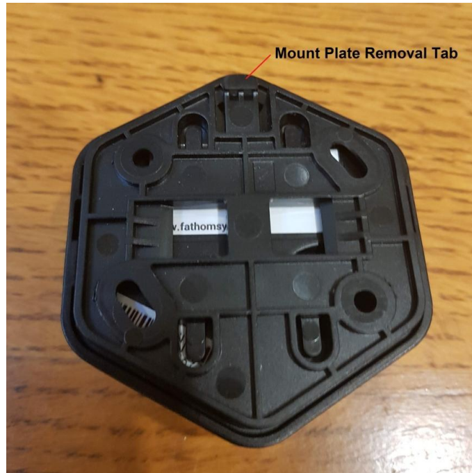
Figure 64 - wTag with Mount Plate Installed
