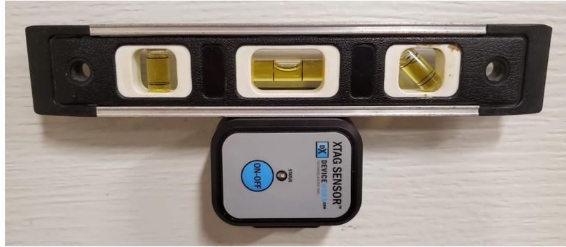
Next, press the CAL ACC-Y button to perform the calibration and store calibration data within the xTAG. A confirmation pop-up message will be displayed when the calibration is complete.
